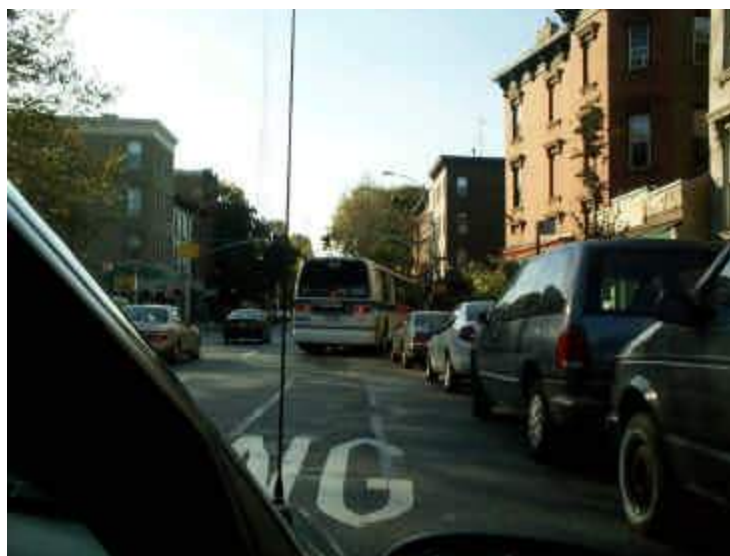
Figure 7.6 Court Street: Buses partially blocking the travel lane encourage vehicles to straddle two lanes while passing
